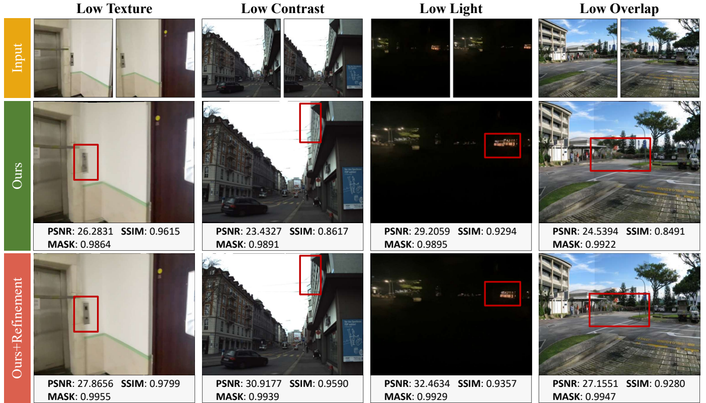
Fig. 7: Challenging examples characterized by low-texture, low-contrast, low-light, and low-overlap. The 1 st to 3 rd rows respectively show the inputs and the results of our method before and after fine-tuning, with red boxes highlighting the performance improvements from fine-tuning.
