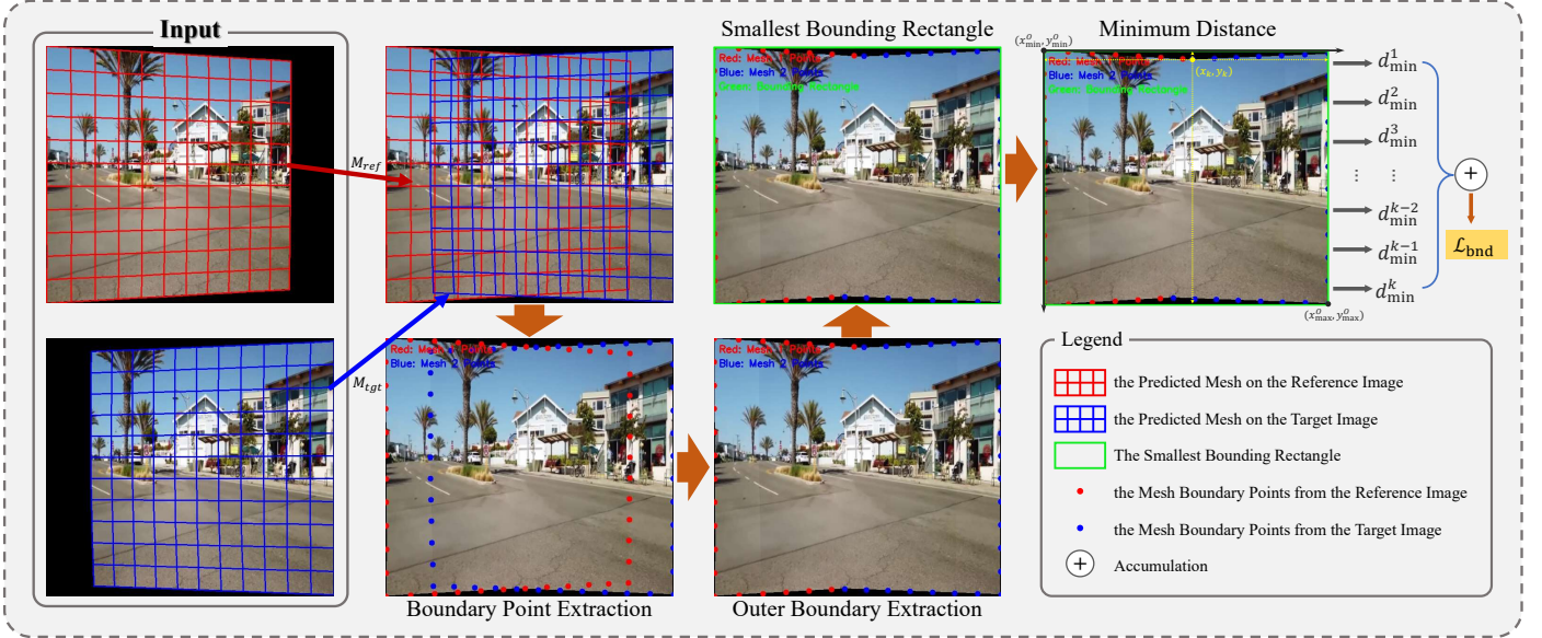
Fig. 2: Illustration of the boundary loss. We take the predicted meshes of the reference image and the target image as input, and then compute the boundary constraint by calculating the sum of the minimum distances from the outer boundary points of the stitched image to the minimum bounding rectangle (marked in green). As the legend shows, the red and blue meshes represent the predicted meshes of the reference and target images, respectively, and the red and blue points are the extracted vertices from those predicted meshes.
