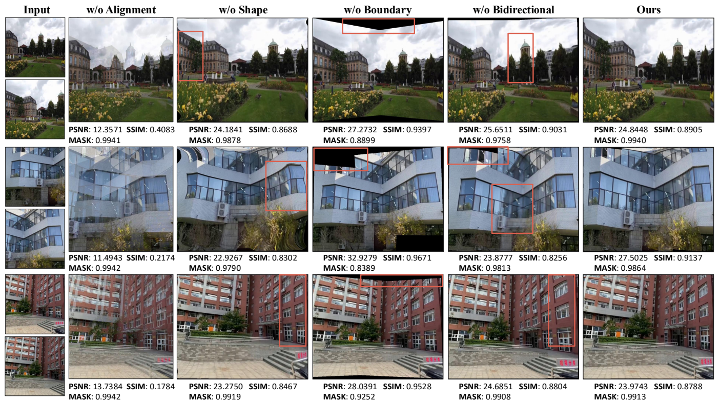
Fig. 8: The stitching results of the ablation study on the UDIS-D dataset [19]. Columns 2 to 5 show the stitching results obtained without alignment, shape preservation, boundary constraints, and bidirectional decomposition, respectively. The last column presents our results with all constraints incorporated, while red boxes indicate artifacts in the results obtained without these key constraints.
